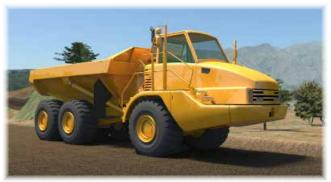
Articulated haul trucks covered in this guide are off-highway trucks and diesel-powered mechanical drive.
