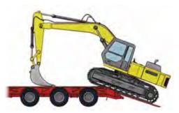
8. Raise the bucket until it just clears the deck and position the machine on the vehicle to make sure the load is correctly shared by the wheels.
