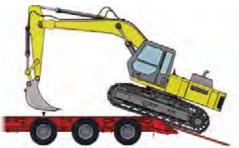
9. Move the bucket close to the operator's platform and lower the boom down until the boom weight is resting on the deck.
