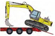
9. Move the bucket close to the operator's platform and lower the boom down until the boom weight is resting on the deck.
