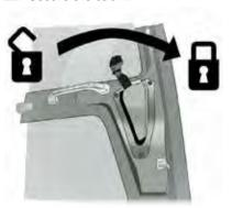
12. Secure the machine to the vehicle.
