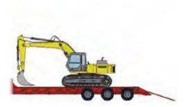
7. As the machine rocks over onto the deck raise the bucket slowly to prevent the machine coming down hard onto the deck.
