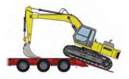
8. Raise the bucket until it just clears the deck and position the machine on the vehicle to make sure the load is correctly shared by the wheels.
