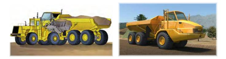
Articulated haul trucks covered in this guide are off-highway trucks and diesel-powered mechanical drive.
