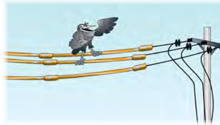
These powerlines have been insulated
