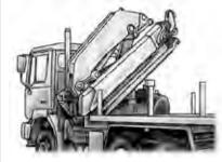
Check for obvious signs of damage on the boom / jib or crane. Stow the boom according to manufacturer's specifications.
