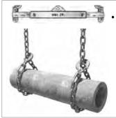
SLING Type: 2 legged vertical load choked chain sling attached to a spread beam with 2 anchor points
