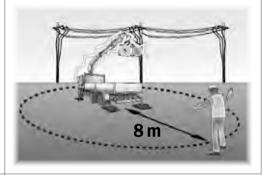
**Do not** use the crane until it has been checked out.
