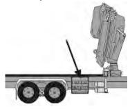
Make sure outriggers / stabilisers are retracted and stowed. Use load restraints where needed.
