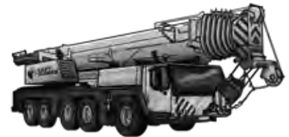
Mobile slewing crane
