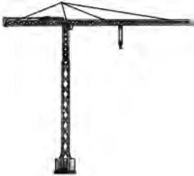
Hammerhead tower crane
